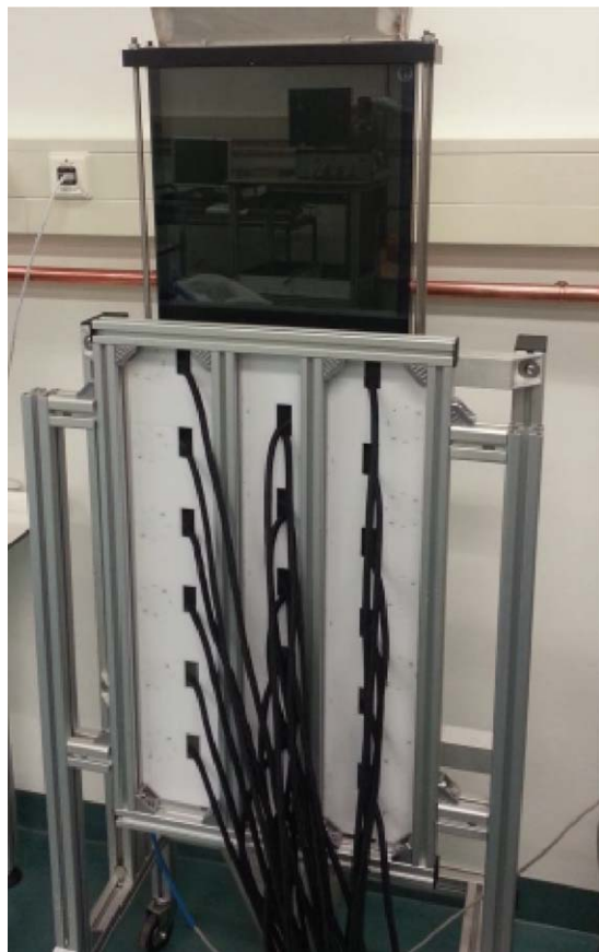
Figure 2. MPT sensor array and pseudo 2-D fluidized bed setup.
